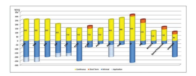
The graph indicates generic minimum and maximum temperatures for different polymers in Yellow and Blue respectively; the printed figured on each is the maximum continuous temperature possible. The extended range in Orange and Grey demonstrates that the polymers temperature envelope can be increased for specific applications and/or for short term use.
